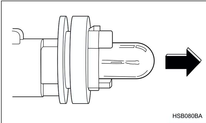
7. Pull the bulb out of the socket. Install a new bulb.
