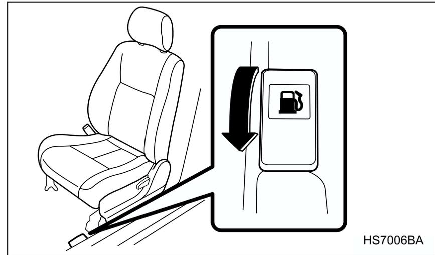
1. To open the fuel filler lid, pull the lid release lever up.
