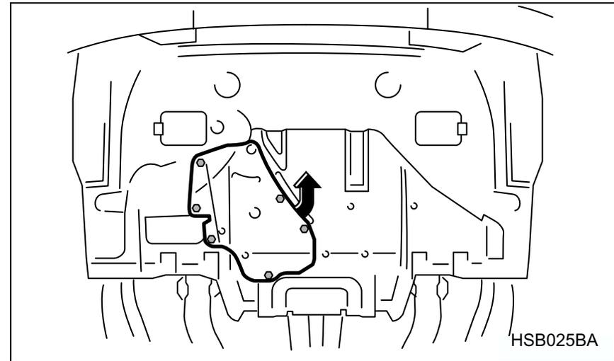
4. Open the access cover by removing the six clips and turning the access cover counterclockwise. The drain plug and oil filter will be exposed.
