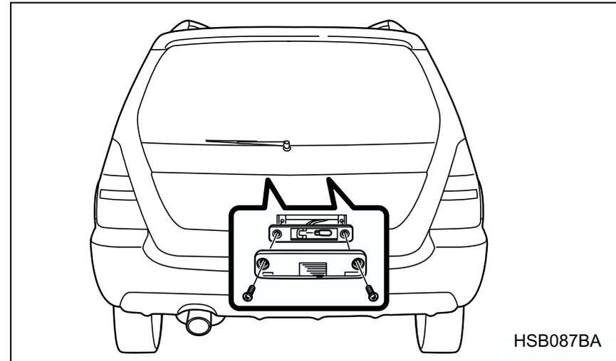
1. Remove the mounting screws using a phillips screwdriver.
