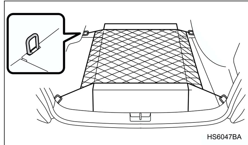
The cargo area is equipped with four tie-down hooks so that cargo can be secured with a cargo net or ropes.
