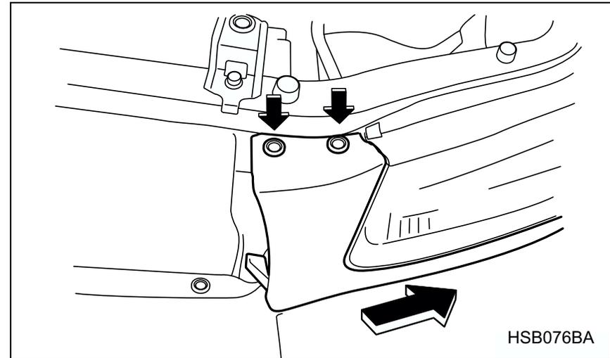
2. Remove the grille side cover by undoing the two clips and sliding the grille side cover toward the headlight.
