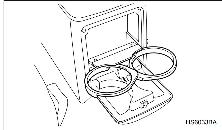
A dual cup holder is located at the back of the center console. To use the cup holder, open the lid by pulling its upper edge.
