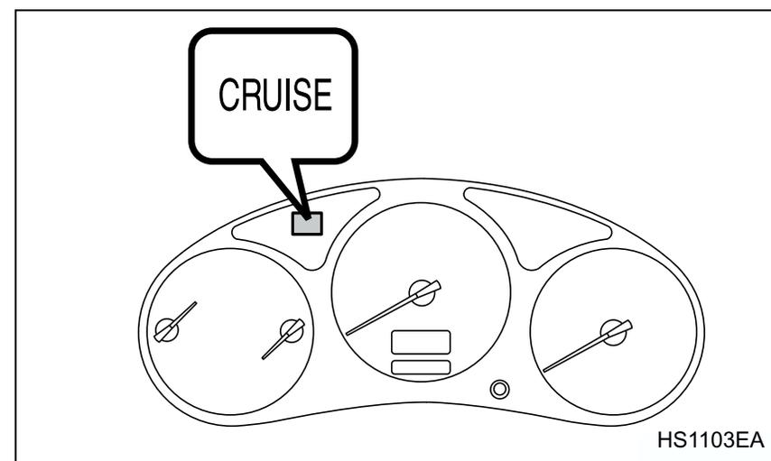
1. Push the "CRUISE" main switch. The indicator light on the instrument panel will come on.
