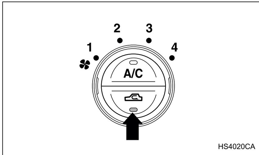
Select air flow by pushing the air inlet selection switch “
