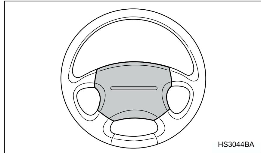
To sound the horn, push the horn pad.
