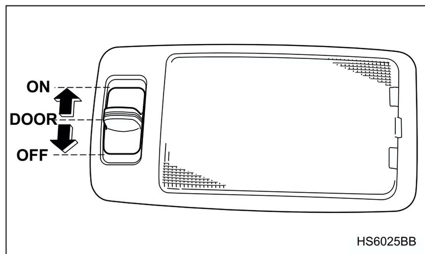
The dome light switch has three positions:
