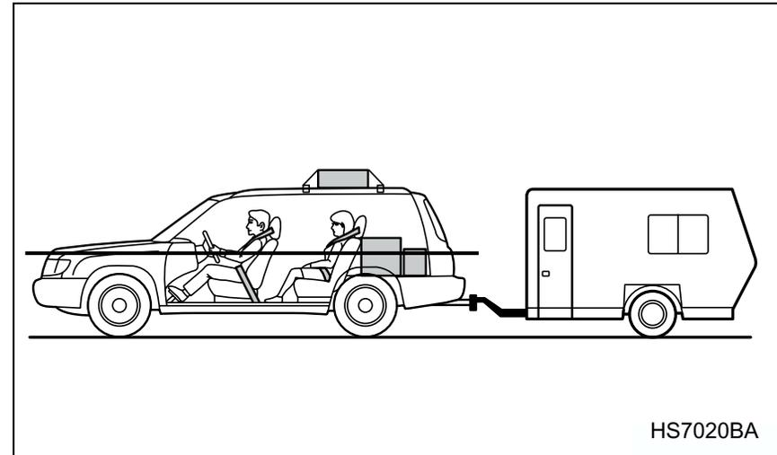
Owing to the self-leveling suspension, the vehicle body is adjusted to the proper position after several drive trips, even if the rear of the vehicle is lowered by loaded cargos or a coupled trailer.
