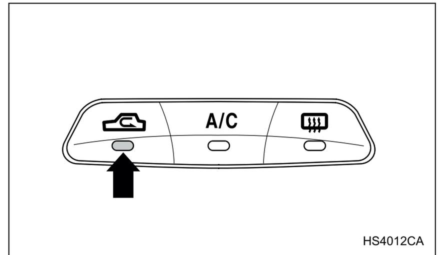
**ON position (Recirculation):** Interior air is recirculated inside the vehicle. Push the air inlet selection button to the ON position. The indicator light will come on.
