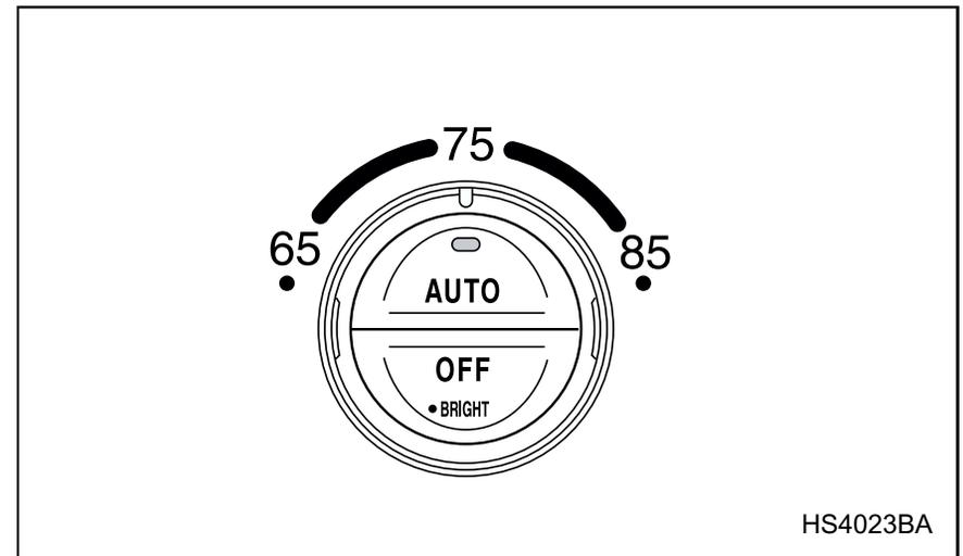
When the “AUTO” switch is pressed, the indicator light on the switch illuminates, indicating that the Automatic Climate Control system is operating in the automatic mode. In the automatic mode, the system maintains the desired cabin air temperature (this is set using the temperature control dial) by automatically controlling the fan speed, air flow mode, air inlet selection, and air conditioner compressor operation.
