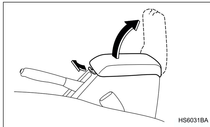
To open the lid, pull up the lock release. If the console lid is fully opened when a large cup is put in the rear passenger's cup holder, the lid may hit the cup and beverage may be spilled.
