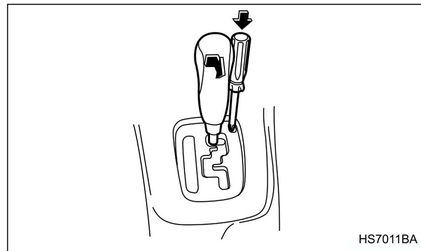
4. Insert the screwdriver into the hole.
