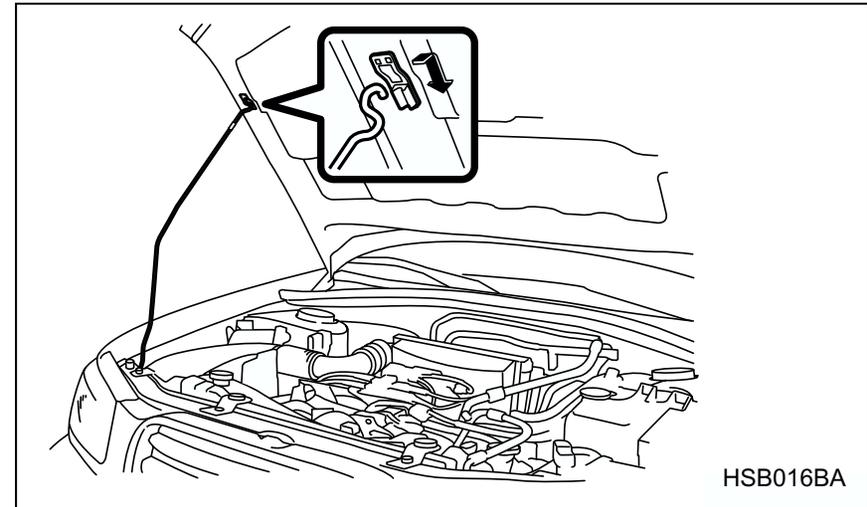
Lift up the hood, release the hood prop from its retainer and put the end of the hood prop into the slot in the hood.
