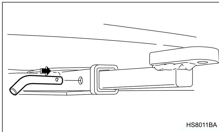
2. Insert the hitch pin into the hole on the hitch receiver
