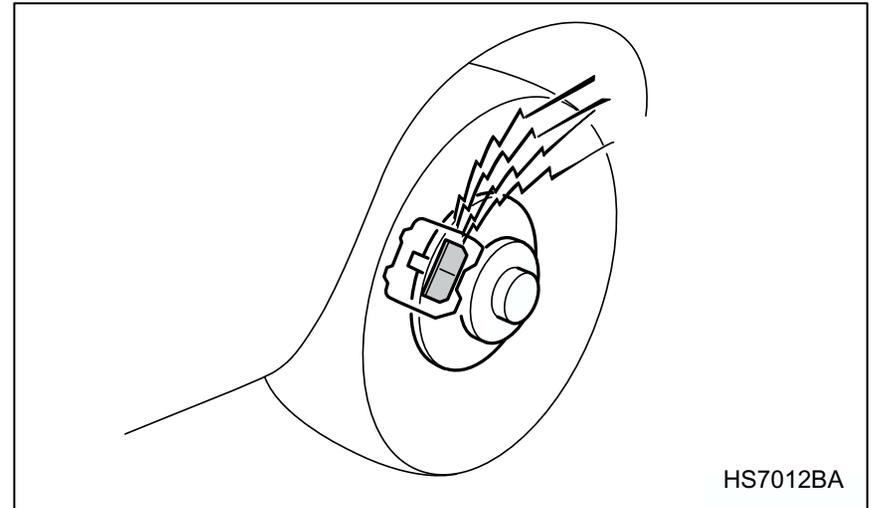
The front disc brakes and the right rear disc brake have an audible wear indicators on the brake pads. If the brake pads wear close to their service limit, the wear indicator makes a very audible scraping noise when the brake pedal is applied.
