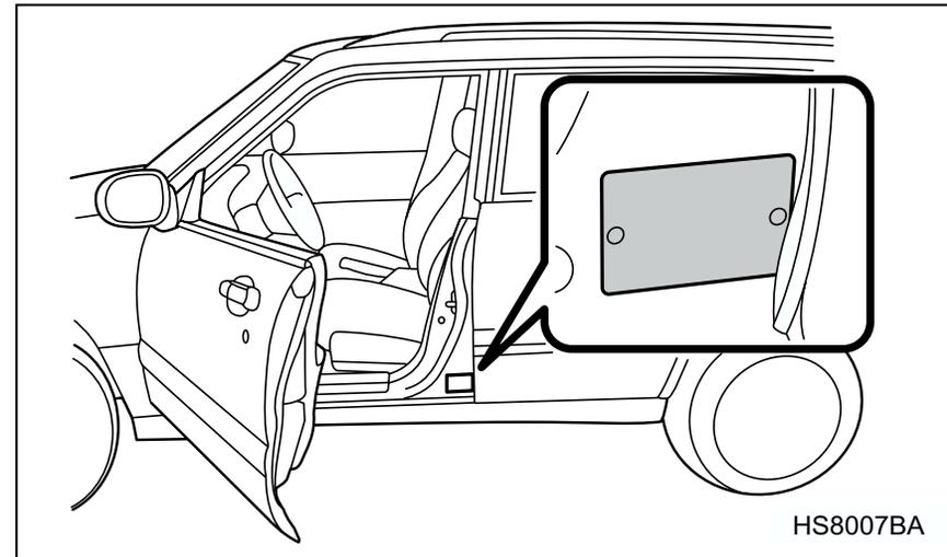
The certification plate attached to the driver's side door jamb shows GVWR (Gross Vehicle Weight Rating) and GAWR (Gross Axle Weight Rating).
