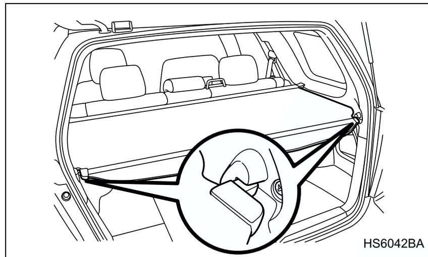
To extend the cover, pull the end of the cover out of the housing, then insert its hooks into the catches as shown. To rewind it, unhook it from the catches and it will rewind automatically. You should hold on to the cover and guide it back into the cover housing while it
