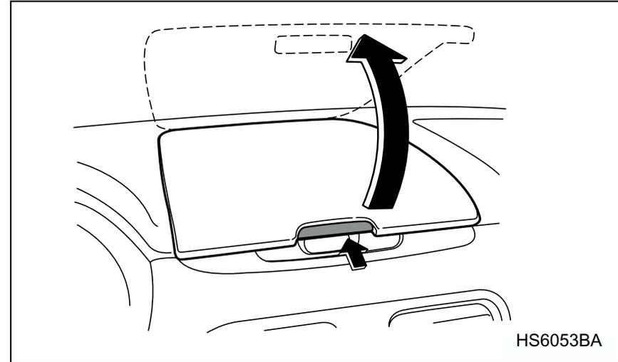
To open the dashboard compartment, push the button on the lid and the lid will automatically open. Be sure to close the compartment fully before driving.
