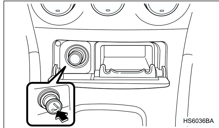
The cigarette lighter operates only when the ignition switch is in the "ON" and "ACC" positions. To use the cigarette lighter, push in the knob and wait a few moments. It will automatically spring up when ready for use.
