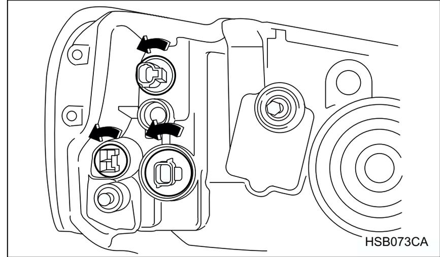
6. Remove the bulb socket from the headlight assembly by turning it counterclockwise.
