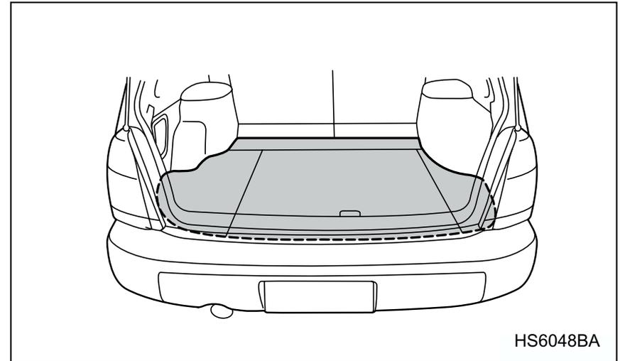
There are four storage trays underneath the floor of the cargo area. They can be used to store small items.
