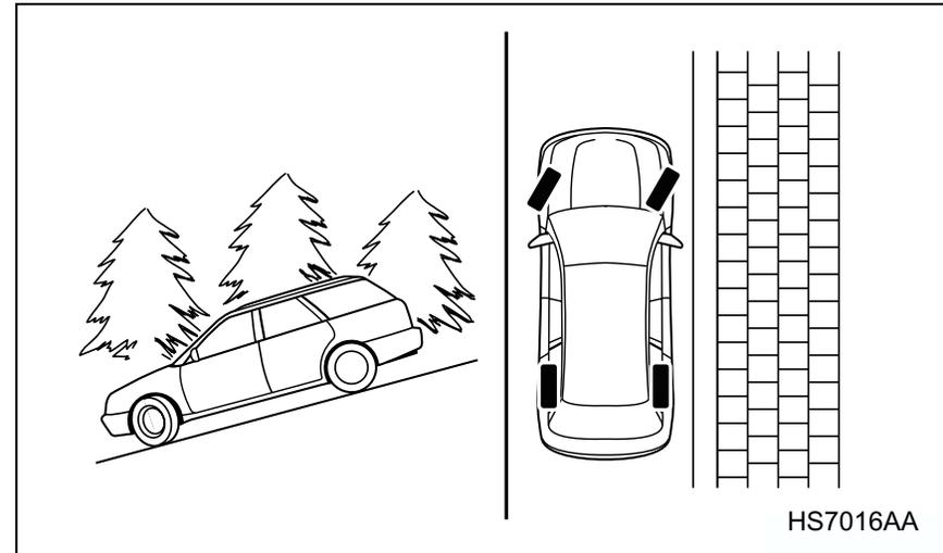
When facing downhill, the front wheels should be turned into the curb.
